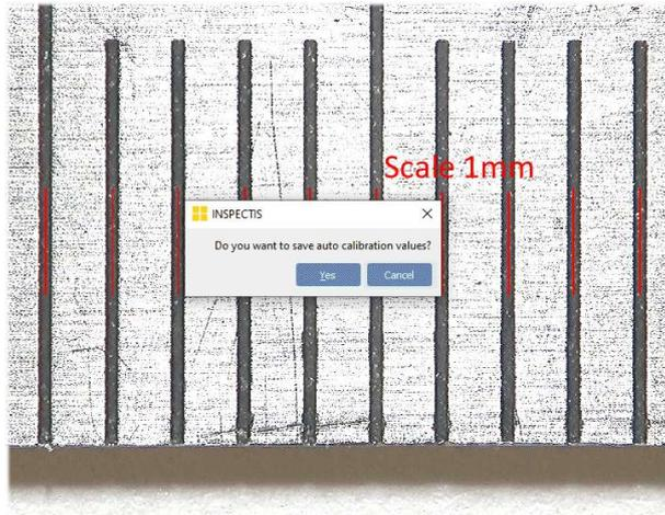
If you wish to Auto calibrate several magnifications within a specific zoom range, select "Auto calibrate zoom range" checkbox and enter the "Upper zoom limit". Software will scan and calibrate all magnification within specified zoom range. Notice Auto calibration of zoom range is not available for Inspectis 5MP Cameras (BGA Inspection).
