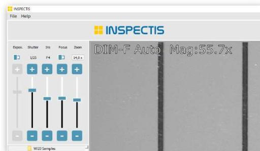
Distortion Correction and Reference Scale are also activated automatically by software.
