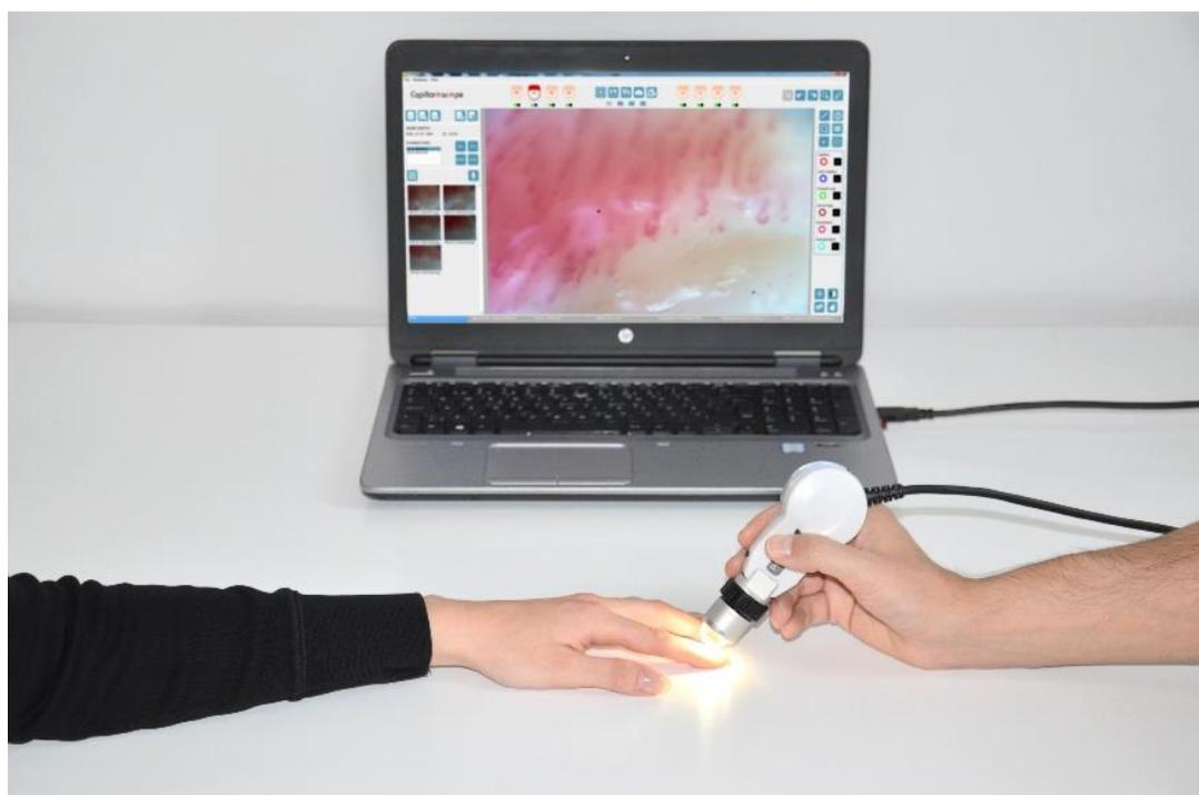
Focusing can be fine-tuned by adjusting the focusing ring or by angling the device towards/backwards relative to the patients nailfold.
