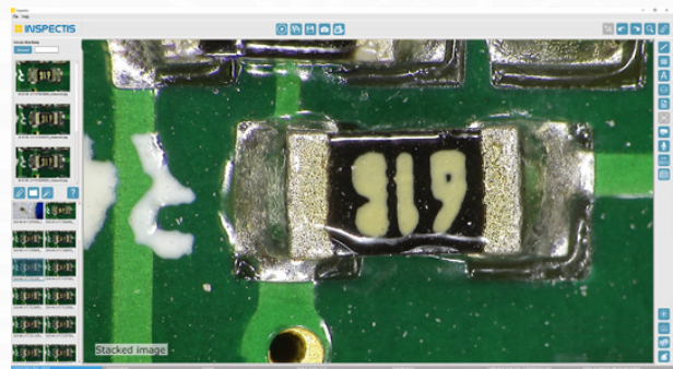
Resistor, focus stacked in INSPECTIS® ProX
