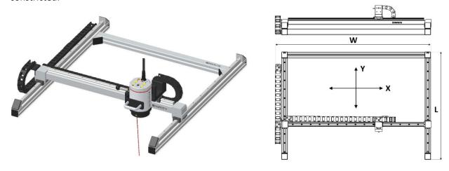
Comprised of custom cut linear guiding system mounted on high density ESD protected 40x40mm or 30x30mm aluminium profiles for smooth and stable XY-travel of digital camera. The system is fitted with mounting brackets to allow the correct setting of working distance during installation in the user's rack system. 4-direction tilt unit, Z-extender bracket and camera grip handle are available for XY-travel Stand as extra accessories.
