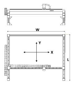
Comprised of custom cut linear guiding system mounted on high density aluminium profile for smooth and stable XY-travel of digital camera. The height of the linear guide can be adjusted and set for desired working distance of the Digital Microscope. 4-direction tilt unit, Camera grip handle, and Z-extender brackets are available for XY-travel Stand as extra accessories.
